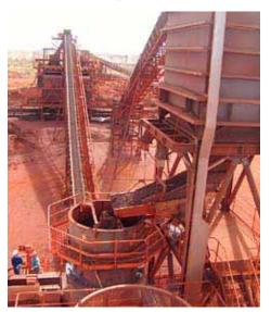
The Sandvik CH880 cone crusher in an Australian open-cast mine.
